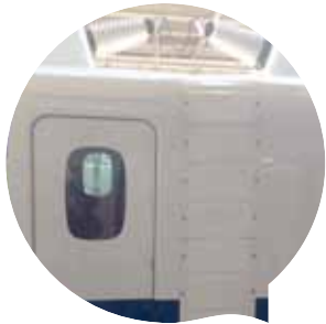
TO REDUCE THE 'DRAG' EFFECT OF THE SEPARATION BETWEEN CARRIAGES, SHINKANSENS ARE NOW FITTED WITH THESE HIGH TECH DIVIDING SHROUDS
